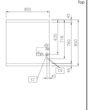
Electric Supply voltage: 400 V/3N ph/50/60 Hz Electrical power, max: 12 kW **Key Information:** 100 °C **Working Temperature MIN:** Working Temperature MAX: 450 °C External dimensions, Width: 800 mm External dimensions, Depth: 850 mm External dimensions, Height: 250 mm Net weight: 120 kg Configuration: One-Side Operated;Top Front Plates Power: 3 - 3 kW **Back Plates Power:** 3 - 3 kW Solid top usable surface 670 mm (width): Solid top usable surface
